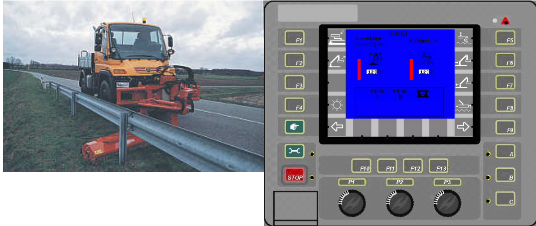
Figure 7.6: Marginal strip mower (“RSM 13”) and its control desk
