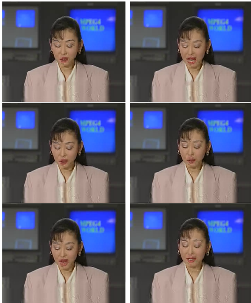
Figure 1.1: Conventional transmission protocol (UDP/IP/IEEE802.11b) gives an unacceptable quality. Sample pictures are taken from MPEG4 CIF sequence Akiyo that was transmitted over four IEEE802.11b hops.
