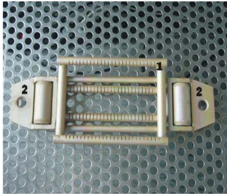
Figure (3-2): The carrier (1) and the boat (2) used to carry the wafers into the tube
