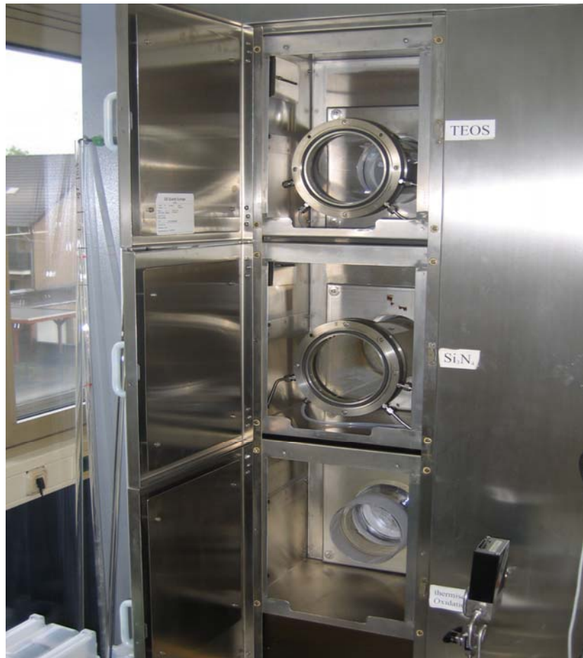
Figure (3-1): 3-zone-oven used to produce \text{SiO}_2 by thermal oxidation, TEOS decomposition, deposition of \text{Si}_3\text{N}_4 and \text{SiON} layers by LPCVD
