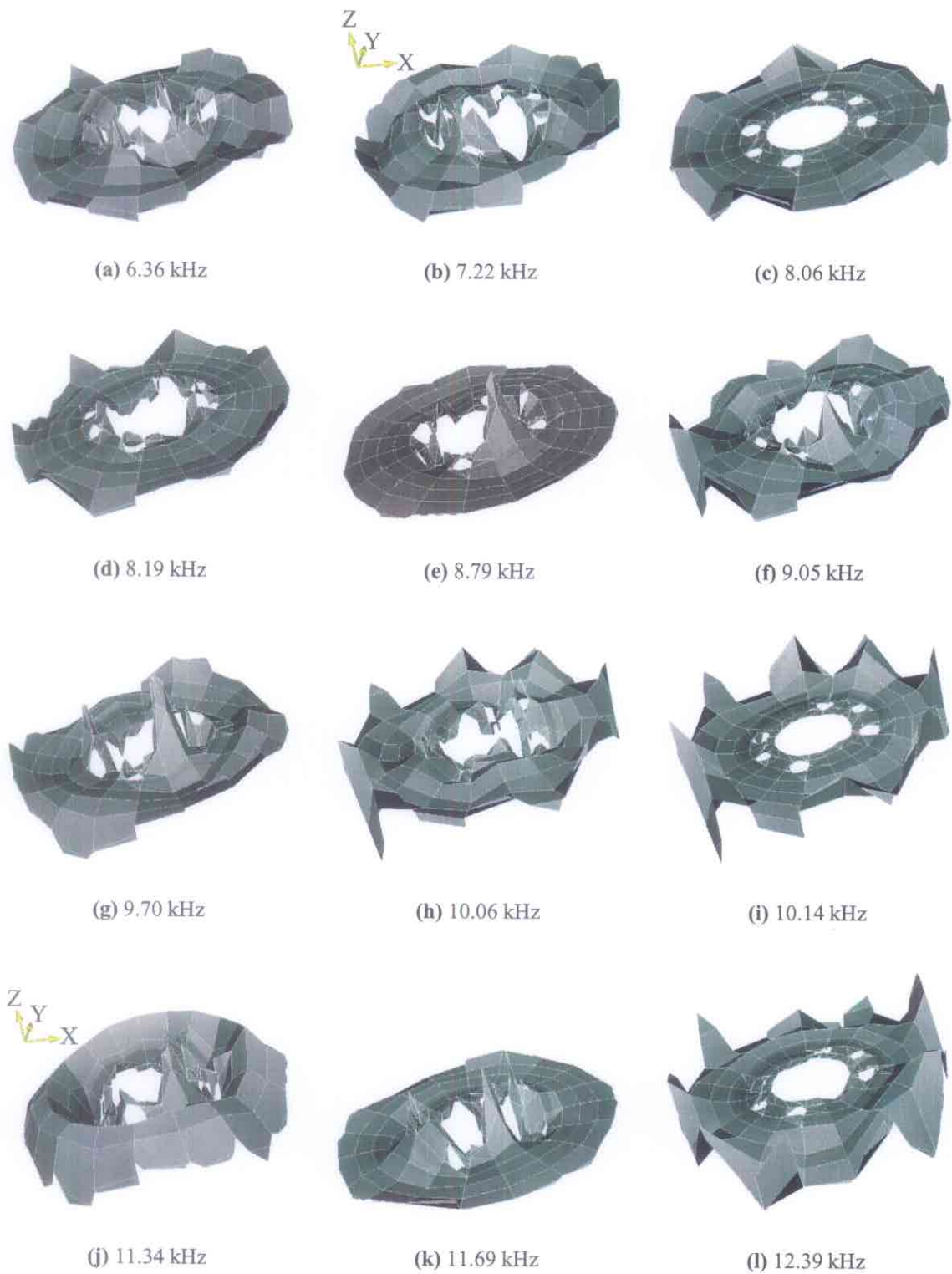
Figure B.2.: Disc out-of-plane deflection shapes in the frequency range 6.3 kHz to 12.5 kHz
