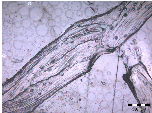
Figure 4.28: Rupture of a trabecula joint of a bovine vertebral specimen, load axis is in vertical direction, specimen has been embedded and sectioned (LM).
