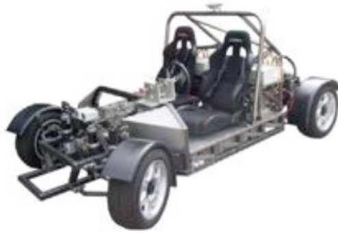
Figure 2.18: Stanford steer-by-wire test vehicle P1, LAWS ET AL. (2005, [70])
