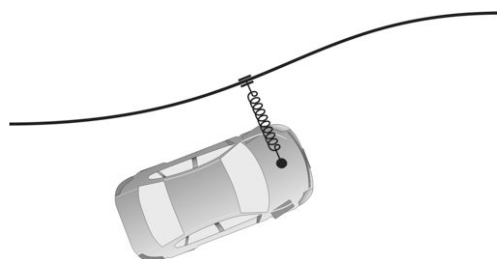
Figure 1.4: Potential field based vehicle guidance control
