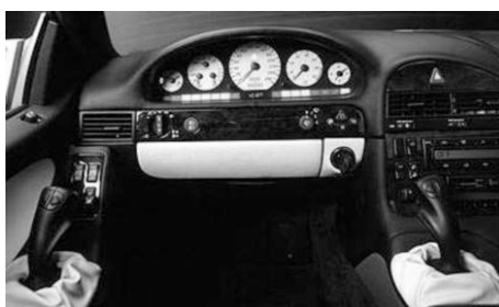
Figure 1.3: DaimlerChrysler "SideStick" according to ZEILINGER (2005, [127])
