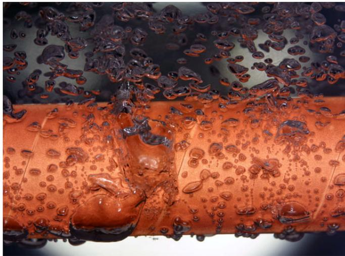
Figure 4.1.46: Boiling of FC-3284 on A425 at  $p = 0,5 \text{ bar}$ ,  $q = 3 \text{ kW/m}^2$ .
