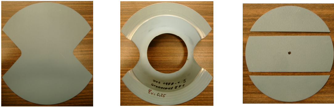
Fig. 22. Preparation of plane strain formed samples for in-situ Raman / EIS analysis
