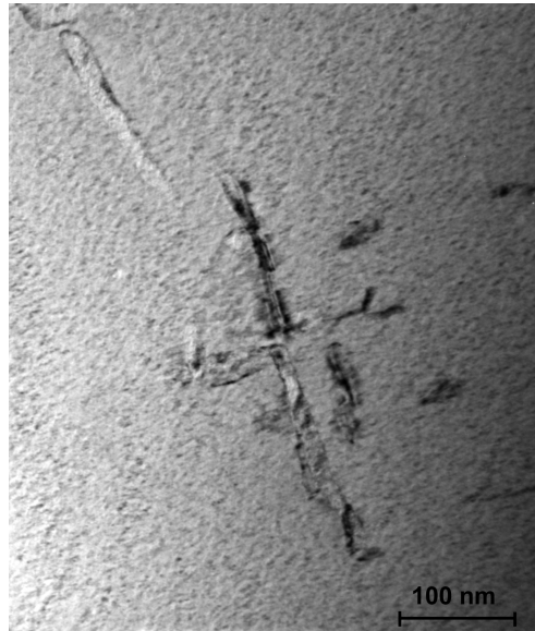
Figure 4.10: Bright field image showing the microstructure of Type I trained \text{Co}_{49}\text{Ni}_{21}\text{Ga}_{30} [001]-oriented single crystals.
