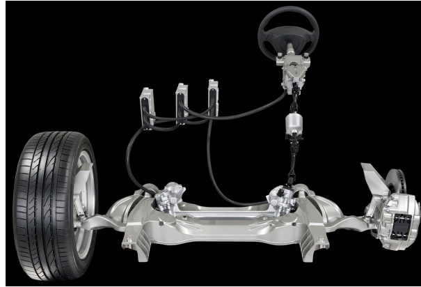
Figure 1.3: CAD model of upcoming Steer-By-Wire system from Nissan (Image: Nissan).
