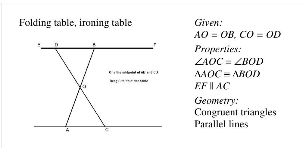
**Abbildung 2.38** – „Mechanical Linkages and their associated Geometry“ (VINCENT 2002, S.133)
