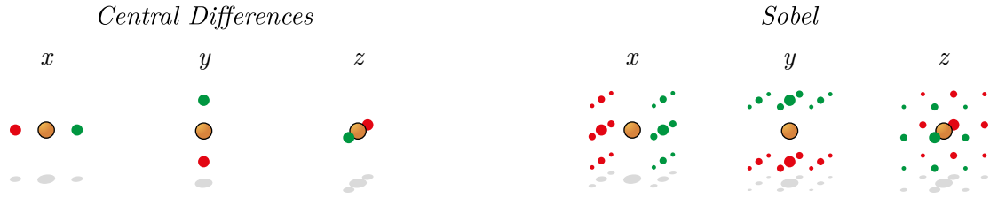
Figure 2.15: Illustration of common sampling patterns for computation of x , y and z component of the gradient. Orange dots indicate the sampling position the gradient shall be computed for. Red and green dots indicate sample positions, at which the volume is sampled to compute the gradient. The size of the dots indicates their weight. The weighted sum of the values at red positions is subtracted from the weighted sum of the values at green positions to determine the x , y , or z component, respectively. Drop shadows help to understand the pattern.
