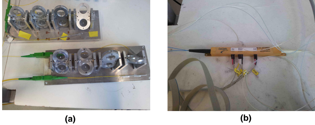
FIGURE A.5: (a) Polarization Controller (b) Celight 90° Optical Hybrid
