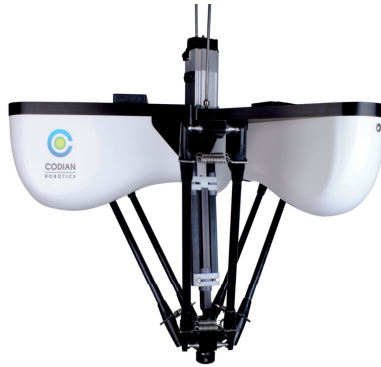
Figure 3.1: D4-500 Delta parallel robot from CODIAN Robotics
