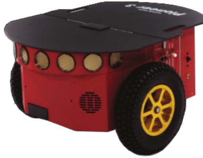
Figure 2.20: A two wheeled differential drive robot model Pioneer P3 DX (from [pio15]).
