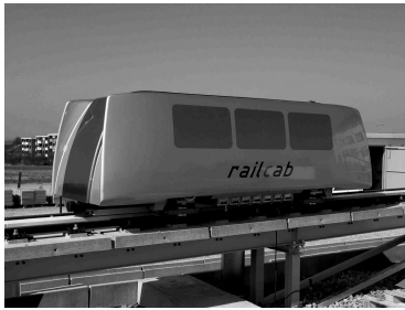
(a) RailCab Prototype in Scale 1:2.5 on Test Track
