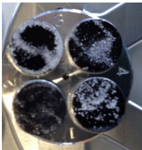
Figure 43: Four different particle samples immobilized on sticky carbon tapes. The carbon pad is dipped in the particle powder and excess particles are removed by means of blowing with a stream of nitrogen. The actual corresponding SEM images are depicted in Figure 4.
