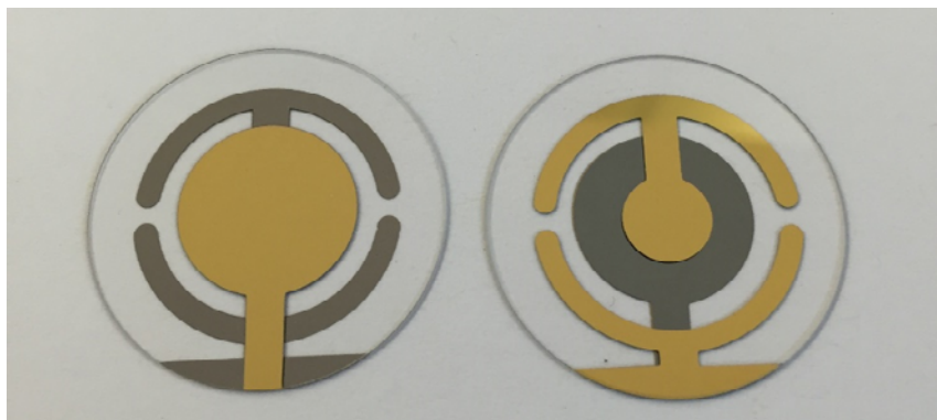
Figure 25: Photograph of the front (left) and back (right) of a typical 1 inch AT-cut QCM crystal with a resonance frequency of 5 MHz featuring a back electrode that is considerably smaller than the front electrode.
