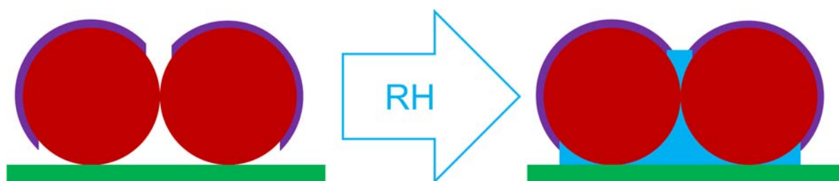
Figure 75: Schematic of the proposed coverage of the organosilane on the particle modified crystal.
