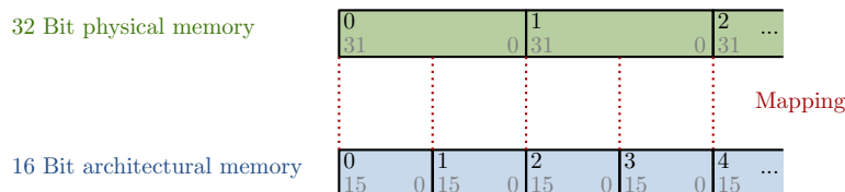
Figure 6.1: A 32 bit wide physical memory and a 16 bit view via an architectural interface.
