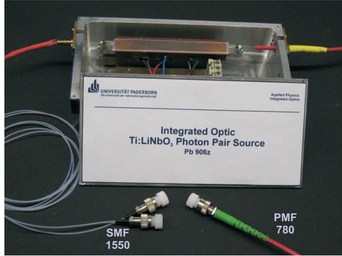
Figure 4.23: Photograph of the packaged and pigtailed device.
