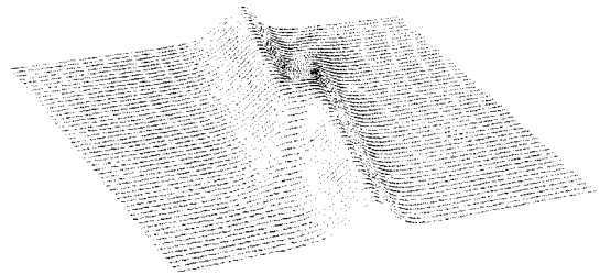
Fig. 2.Bb. Second Decomposition of KdV. Smaller Soliton. c_1=2.56 , c_2=1.08 .
