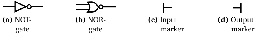
Figure 2.1: A NOT- and a NOR-gate as well as the markers incident to input nodes and output nodes.
