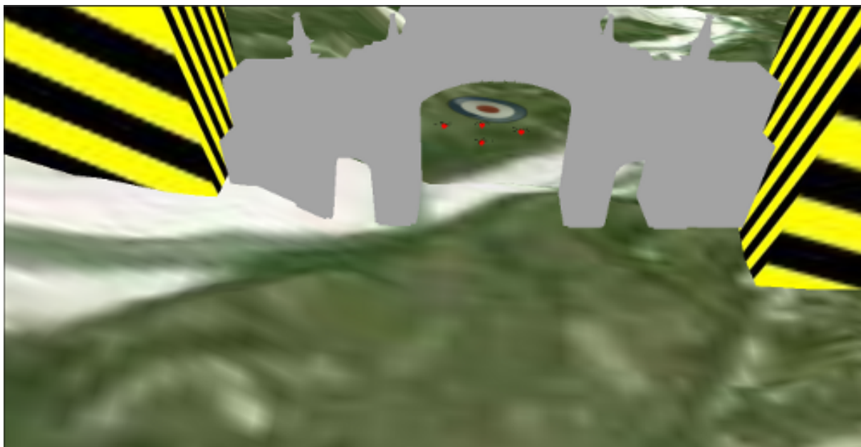
Figure 8.20.: Cutout of an screenshot from the Control Station showing the change of the formation shape conducted by the UAVs to adapt the formation to the environment in order to fly through the small passage given by the triumph arch.
