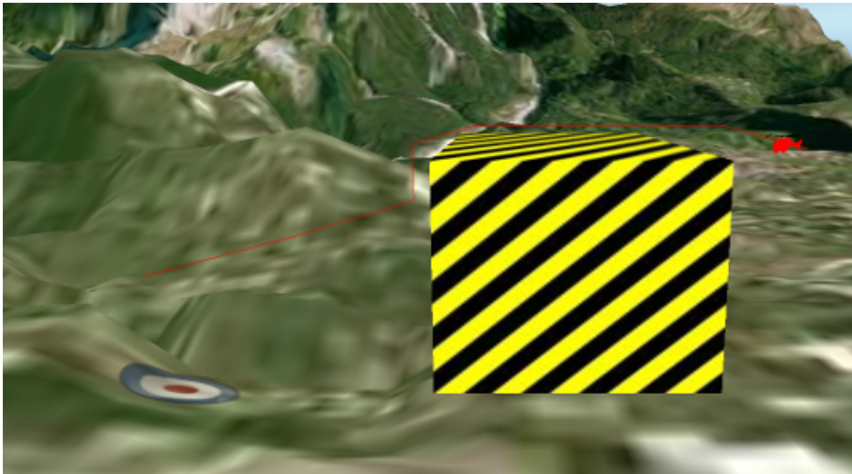
Figure 8.17.: Newly computed trajectory after an obstacle intersected the previously computed UAV path.
