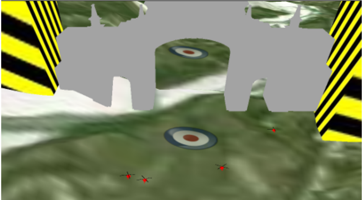
Figure 8.18.: The initial configuration used to show the obstacle avoidance behavior of a UAV formation. The red UAVs are distributed over the environment and have to create a line formation at the target position in front of the triumph arch represented by a ring shaped object.
